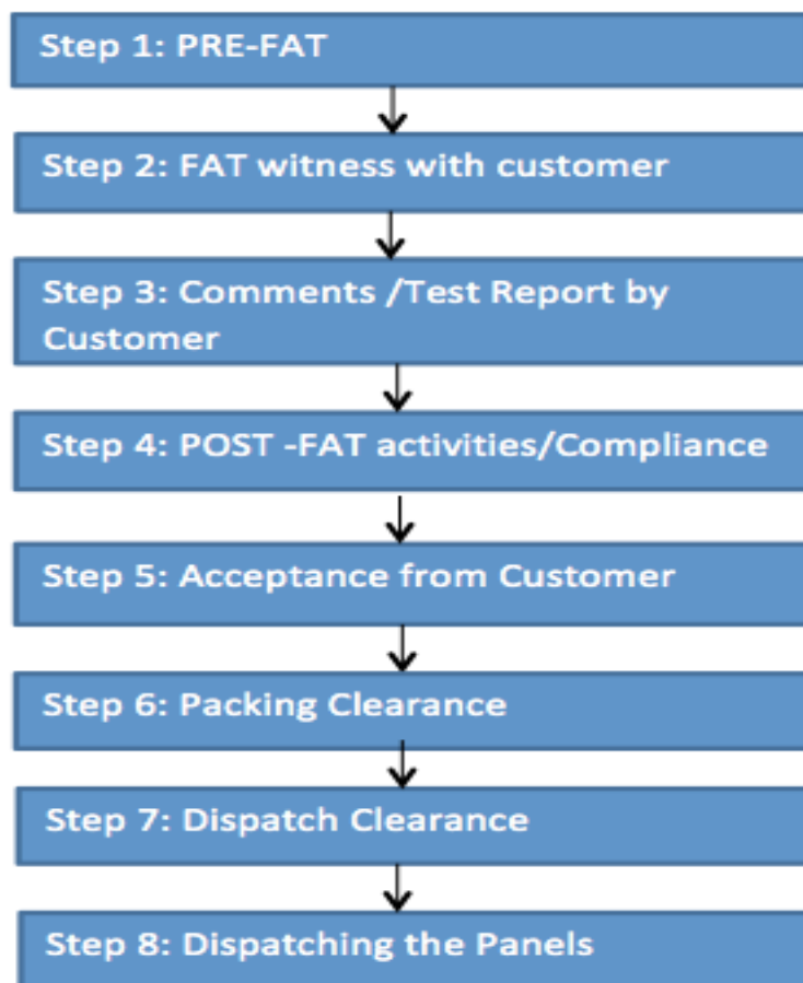
Figure-5 FAT-Quality Control Process Overview
